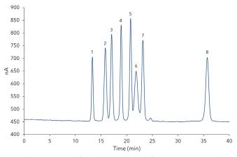
Fig.1 Chromatogram of mixed standard with  $\beta$ =5.00 µg/mL. 1 - saccharose, 2 - glucose, 3 - xylose, 4 - galactose, 5 - arabinose, 6 - mannose, 7 - fructose, 8 - mannitol.
