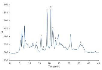
Fig.2 Chromatogram of free hydrocarbon content. 1 - saccharose, 2 - glucose, 3 - xylose, 4 - galactose, 5 - arabinose, 6 - mannose, 7 - fructose, 8 - mannitol.
