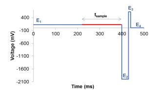
Fig. 4 4-step PAD potential waveform for the detection of monosaccharides and other carbohydrates. The sample detection occurs during the highlighted time period  $t_{sample}$ .
