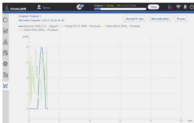
Fig. 8-6 Normalized traces shown in the chromatogram.
