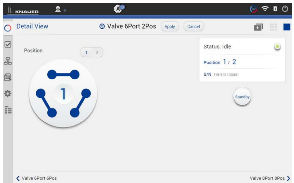
Fig. 5-31 Detail View - Example 6 port 2 position valve
