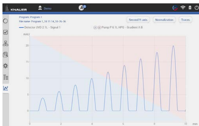
Fig. 8-7 Chromatogram shows UV signal and gradient composition
