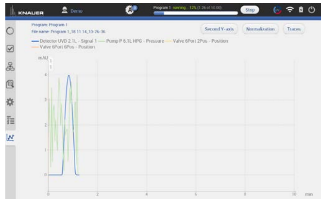
Fig. 8-4 The pressure trace is selected. The y-axis shows the pressure in bar.
