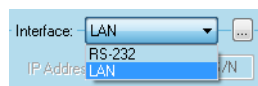
Fig. 50: Available interfaces for detectors MW-1, S 2550, S 2520, 10D, UVD 2.1S, K-2600, CM 2.1S
