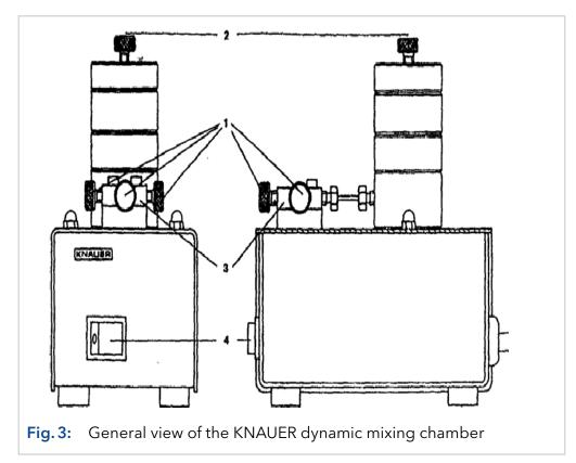
The chamber of the instrument (**Fig. 3**) is composed of four (preparative version three) parts and is set on a housing together with a 4-way 1/16" (1/8") capillary connector, which is used as inlet connection.
