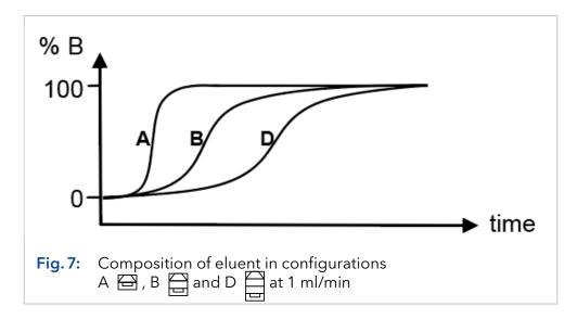
The use of filled intermediate pieces enlarges the static mixing area in addition to the dynamic mixing volume of the lower part. The influence on the response time is obviously whereas on the curve form it is much lower.
