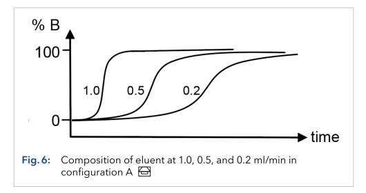
Very similar is the influence of the mixing chamber volume at a given flow rate. The smaller the mixing chamber volume the steeper is the slope of the eluent gradient.
