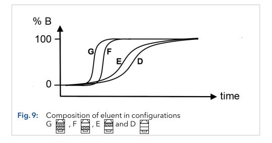
**Note:** Flow rate and volume of the mixing chamber affect the form of the gradient. Mixing chambers from different manufacturers can therefore produce different gradients at the start of the column. The usual details given in the literature for the gradient curve of the controlling instruments are generally not sufficient for reproduction of the same results with other mixing chambers.
