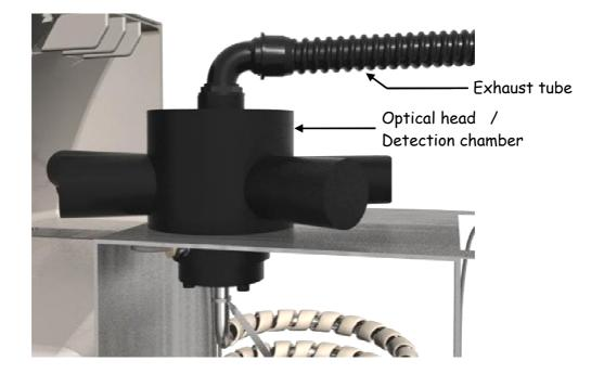
The intensity of the scattered light is a function of the mass of the scattering particles and generally follows an exponential relationship, which is shown in equation 1-1.
