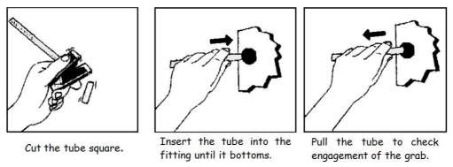
Figure 2-3: Inserting the Gas Inlet Tube
