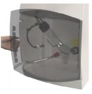
Parafilm<sup> $^{TM}$ </sup> is used to cover various openings inside the compartment, nebulizer and glassware to prevent dust particles from entering the detector during shipment.
