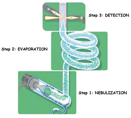
Figure 1-3: Cross-sectional View of the Detector
