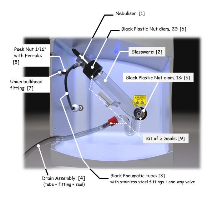
Figure A2-1: Identification of Spare Parts
