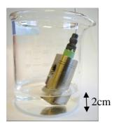
c) Clean the nebulizer for approximately 30 minutes with the solvent, and then replace the solvent with water and clean for an additional 30 minutes.
