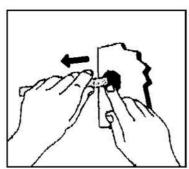
To remove the tube, disengage the grab ring teeth by a simple manual pressure on the push sleeve and withdraw the tube from the fitting.
