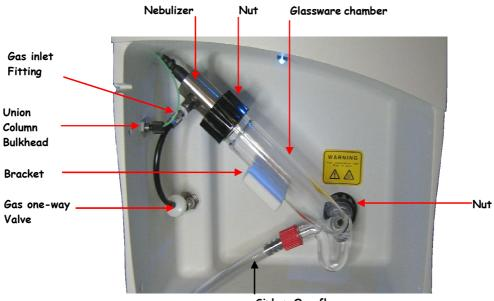
The installed Nebulizer/Glassware Chamber assembly is shown in Figure 2-5.
