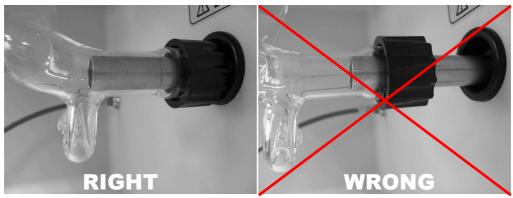
Figure 2-6: Fixing the Glass Chamber
