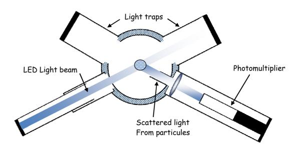
Figure 1-7: Detection Chamber
