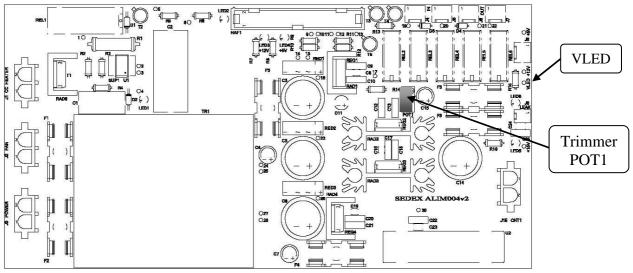
Figure 5-4: The ALIM004V2 Board Lamp Setting
