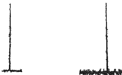
Figure 4-2: Chromatogram with Various Solvent Quality
