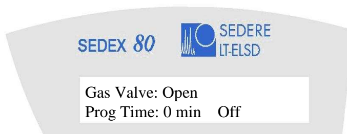
Figure 3-7: The Gas Valve Screen
