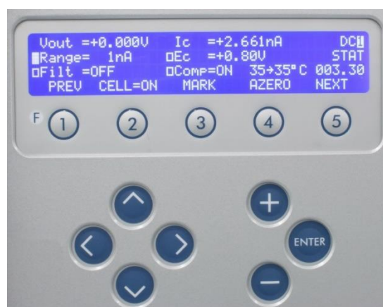
Fig. 6. DECADE Elite keyboard. The cursor is on 'Range' which allows changes using the value buttons '+' and '-'. The 'Enter' button is only used to confirm changes in potential (Ec) and range.
