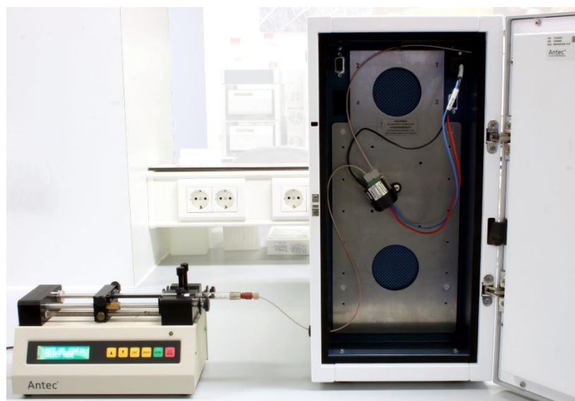
Fig. 40. DECADE Elite scanning voltammetry set-up with a syringe pump.
