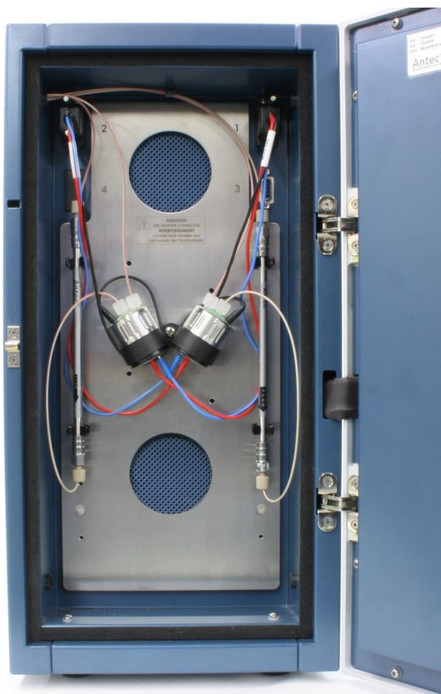
Fig. 13. DECADE Elite with 2 columns and 2 SenCell flow cells for parallel detection.
