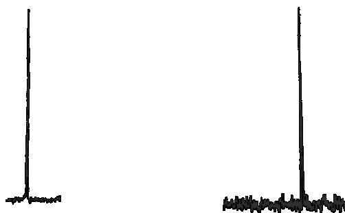
Figure 4-2: Chromatogram with Various Solvent Quality
