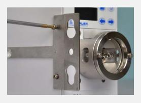
3. Align the guidance clamp with the bore holes of the right-side panel of the AZURA L device and screw it tight with the provided torx screws. Make sure that the upper screw is installed together with the washer.
