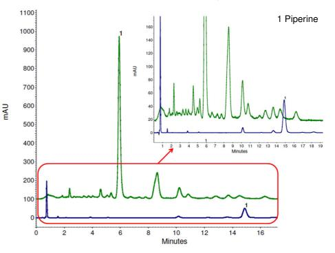
The BlueShell classic phase with a C8 modification was chosen, because it gave the best separation and therewith the best purity control of Piperine. With the first tested BlueShell classic C18 column there was still an impurity eluting at the same time as Piperine. With the C8 modification, retention was much better for Piperine what can easily be seen from figure 6. Piperine elutes comparatively late after about 15 min and is completely separated
