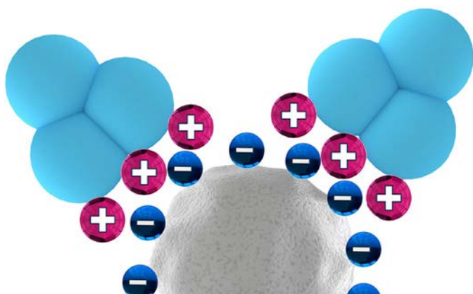
Fig. 1 Principle of cation exchange separation. Proteins with different negative charges bind to the cation exchange resin. By increasing the salt concentration, proteins with a weak negative charge elute first, while at higher salt concentrations, proteins with a strong negative charge elute last.
